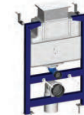
Ancortite 2 in 1 Wall Hung Frame ■ Including pneumatic cistern ■ For use with FP1 and FP2 Flush Plate ■ Adjustment 820 - 1020mm ■ For under window and standard height options ■ Including polystyrene jacket ■ Left or Right turn pan connection option Price Reduction £299 134.DWC
