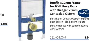
■ Installation height 820mm ■ Flow pressure – 0.1 to 10 bar Operating temperature - 25°C = Flush volume factory setting - 5.8L/3L Flush volume large, adjustment range – 4L/4.5L/6L/7.5L = Flush volume small, adjustment range - 2 to 4L Calculated flow rate - 0.11L/s
